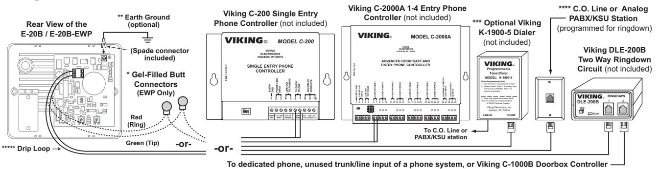
\* **Note:** The gel-filled (water-tight) butt connectors are designed for insulation displacement on 19-26 gauge wire with a maximum insulation of 0.082 inches. Do not strip wires prior to terminating.
