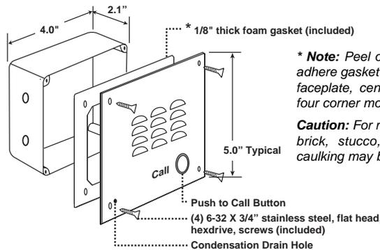
**\* Note:** Peel off paper liner and adhere gasket to the back of the faceplate, centering it over the four corner mounting holes.
