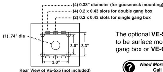
The optional VE-5x5 Surface Mount Box is designed to be surface mounted to a single gang box, double gang box or VE-GNP gooseneck pedestal (right).
