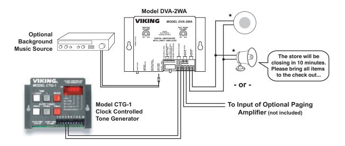
\* **Note:** Up to three 8-ohm speakers may be connected (not included). Viking models **25AE** Paging Horn, **30AE** Ceiling Speaker or equivalent are recommended. For more information, retrieve **Fax Back Document 498**.
