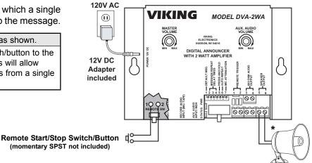
\* Note: Up to three 8-ohm speakers may be connected (not included). Viking models 25AE Paging Horn, 30AE Ceiling Speaker or equivalent are recommended. For more information, retrieve Fax Back Document 498.
